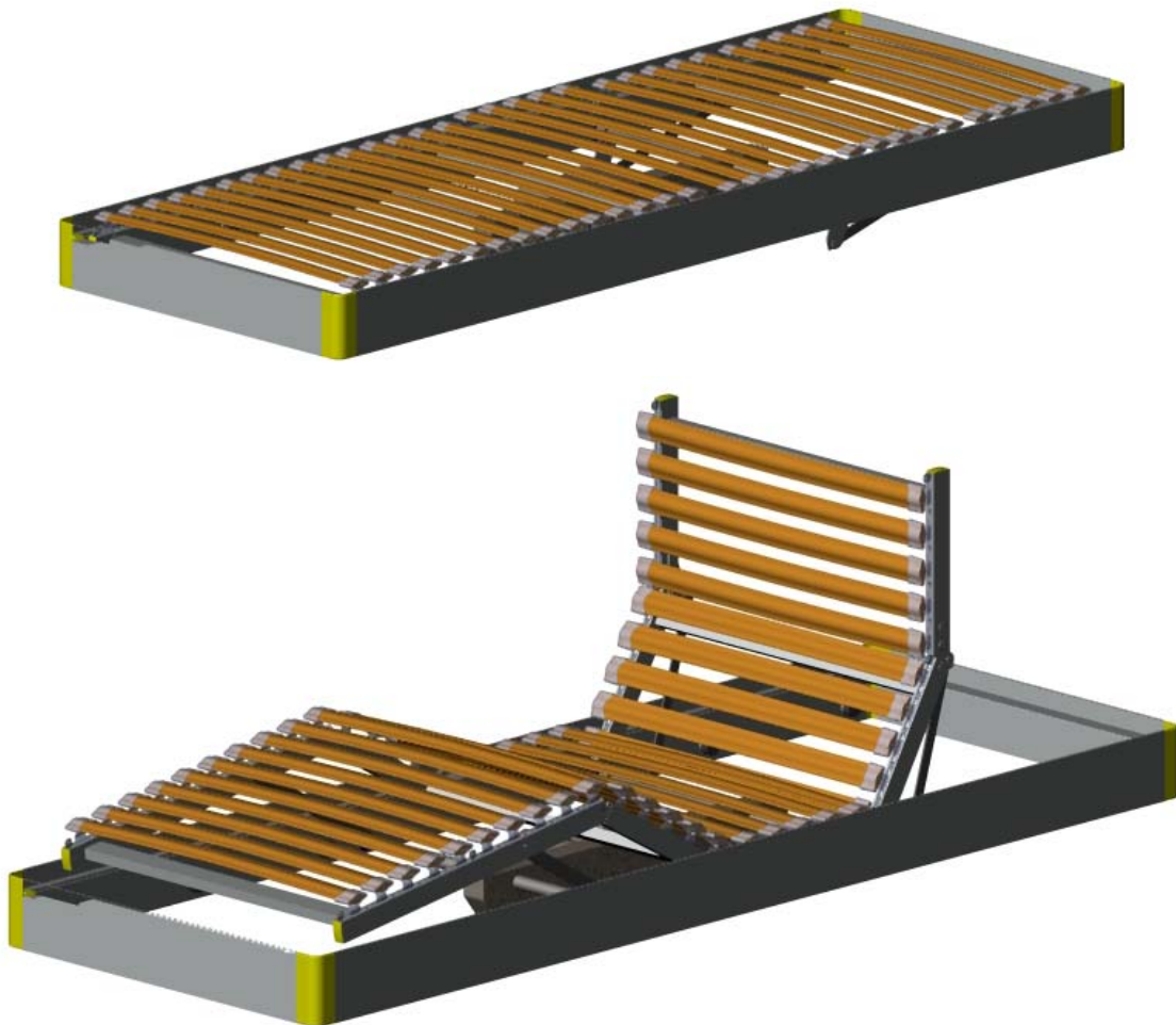
Figure 7-46 A rendered CAD model of the adjustable bed
